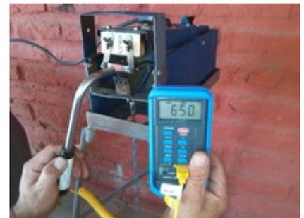
*Pyrometer indicating proper blade temperature of 650°C.*
